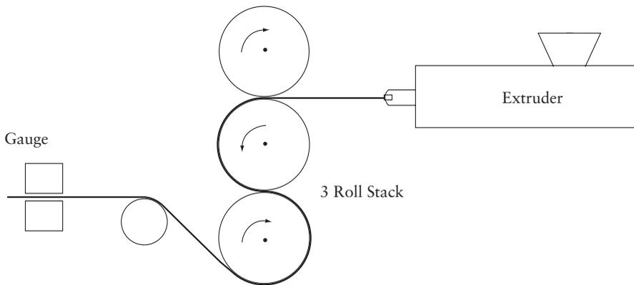
**Figure 4.2** Sheet extrusion line
