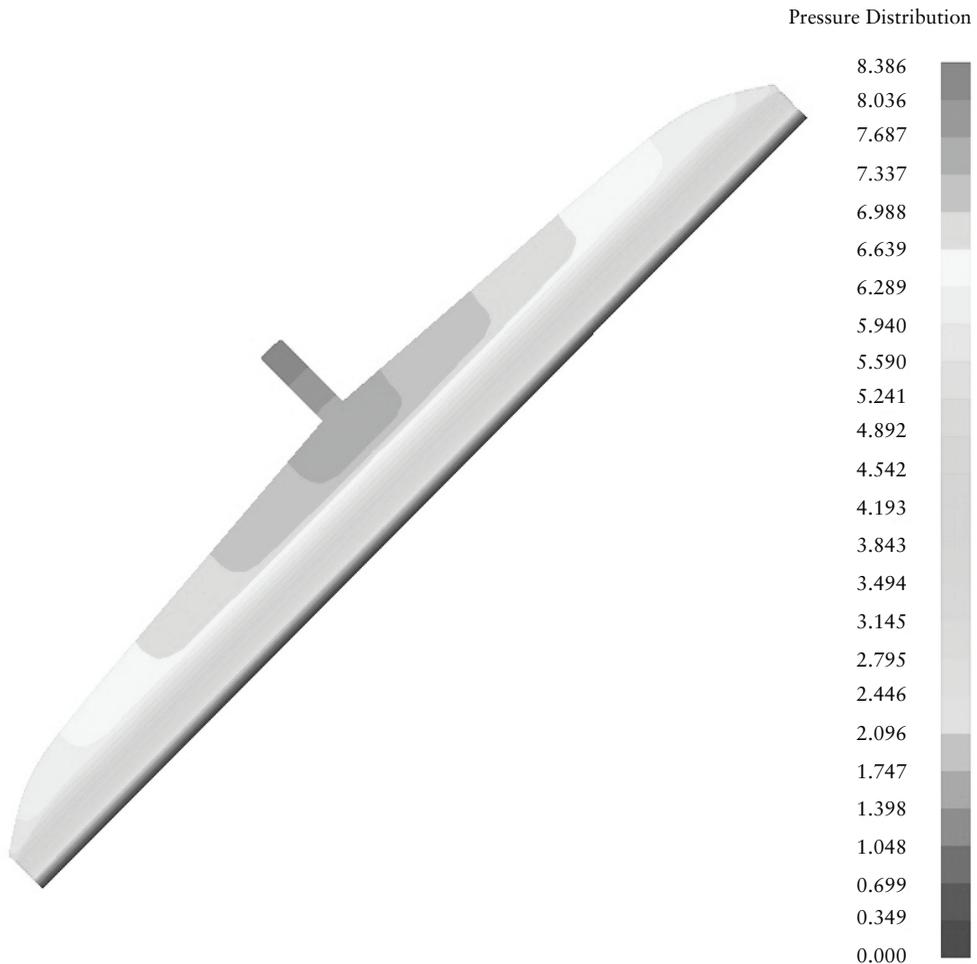
**Figure 4.14** Predicted pressure distribution for the die geometry shown in **Figure 4.12** (200 kg/h)
