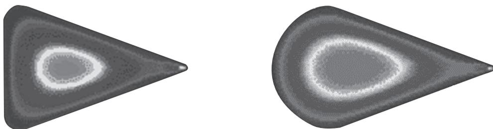
**Figure 4.8** Evolution of the teardrop manifold shape from the older flat back (left) to the modern curved back (right). The highest velocity is in the centre and the lowest on the walls
