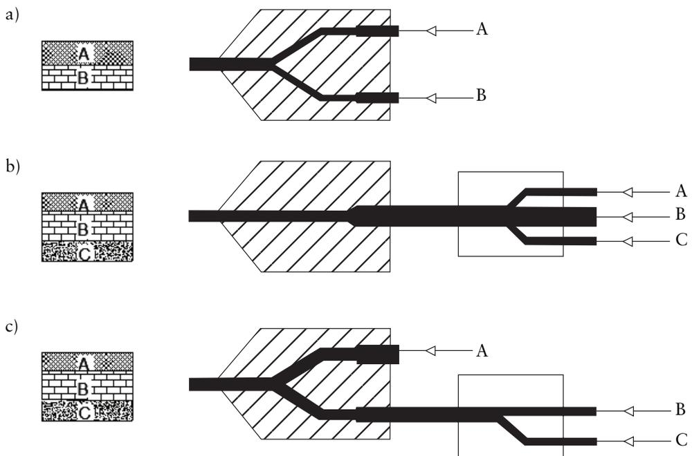
**Figure 4.16** Schematic representation of multilayer extrusion. (a) Multimanifold; (b) feedblock; and (c) combination of feedblock and multimanifold. Adapted from R. Wirtz in *Auslegung von Extrusionwerkzeugen*, VDI Verlag, Düsseldorf, 1996, 72 [7]
