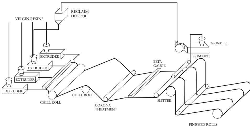
**Figure 4.1** A four-layer cast film line. Adapted from J. Ivey in *The SPE Guide on Extrusion Technology and Troubleshooting*, Eds. J. Vlachopoulos and J. Wagner, Society of Plastics Engineers, Brookfield, CT, USA, 2001, 12.1 [1]
