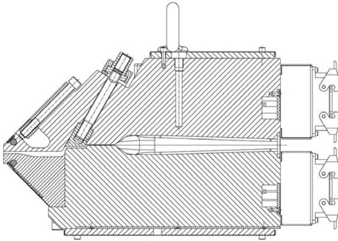
**Figure 4.10** Cross-sectional area of a die having a restrictor bar and a lip adjustment system. Reproduced with permission from EDS GmbH, Kirchdorf, Austria
