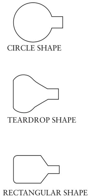
**Figure 4.7** Common types of manifold cross-sections
