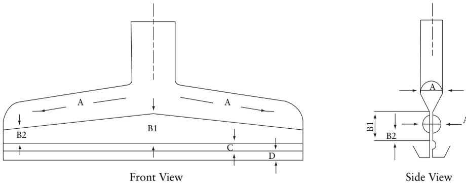
**Figure 4.5** Coat hanger die having a teardrop shaped manifold with a diminishing cross-sectional area from the centre to the sides. A region is the manifold, B1 and B2 are lengths of the preland, C is a secondary manifold and D the land (die lips). Adapted from D.R. Garton in *Film Extrusion Manual*, Eds., T.I. Butler and E.W.Veazey, TAPPI, Atlanta, GA, 1992, p.231 [5]
