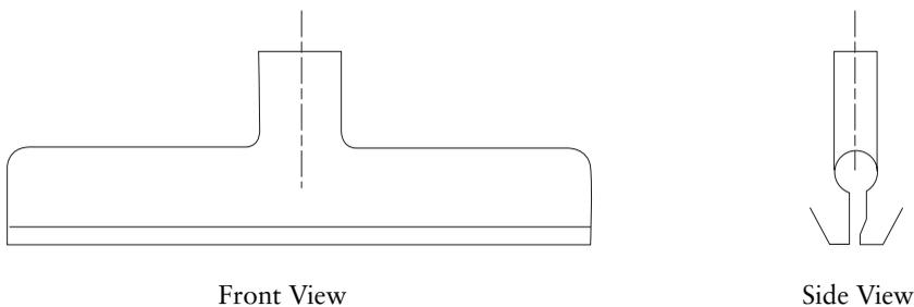
**Figure 4.3** T-slot die with a constant cross-section circular manifold. Adapted from D.R. Garton in *Film Extrusion Manual*, Eds., T.I. Butler and E.W.Veazey, TAPPI, Atlanta, GA, 1992, p.231 [5]
