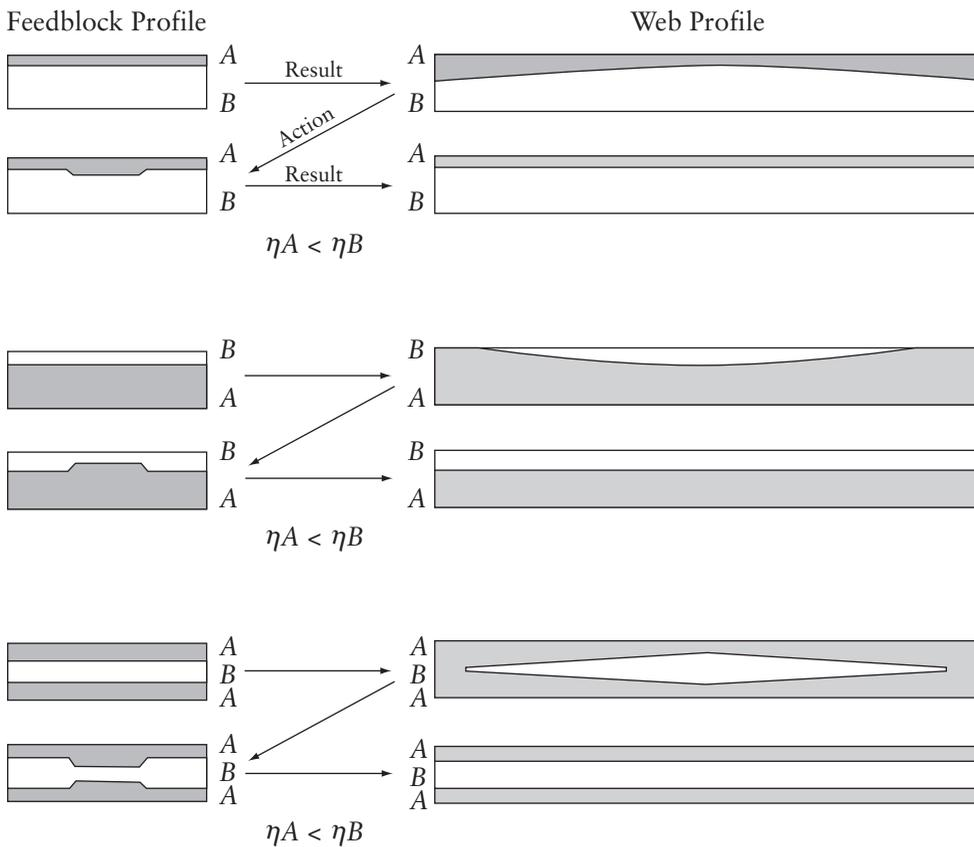
**Figure 4.17** Feedblock profiling and the resultant effects. Adapted from P. Cloeren in *Proceedings of Advances in Extrusion Technology*, RETEC Extrusion Division and the Ontario Section of the Society of Plastics Engineers, Brookfield, NJ, USA, 1993 [33]
