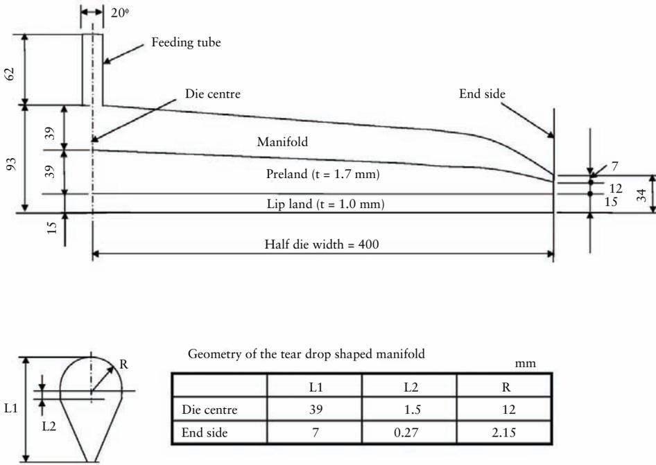
**Figure 4.12** Geometrical specifications of the flat die which was used in the final simulations shown in **Figures 4.13, 4.14** and **4.15**
