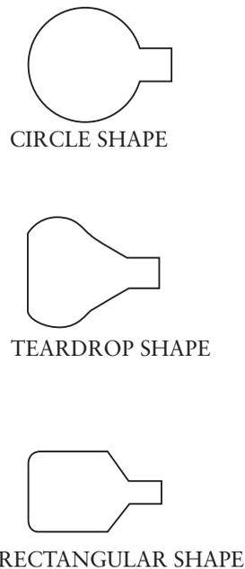
**Figure 4.7** Common types of manifold cross-sections
