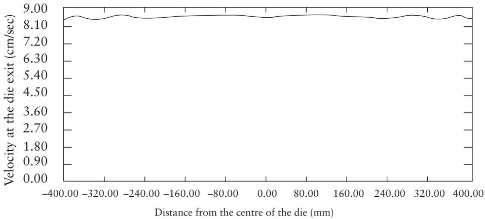
**Figure 4.15** Predicted average velocity distribution at the die exit. Variation  $\pm 1.35\%$
