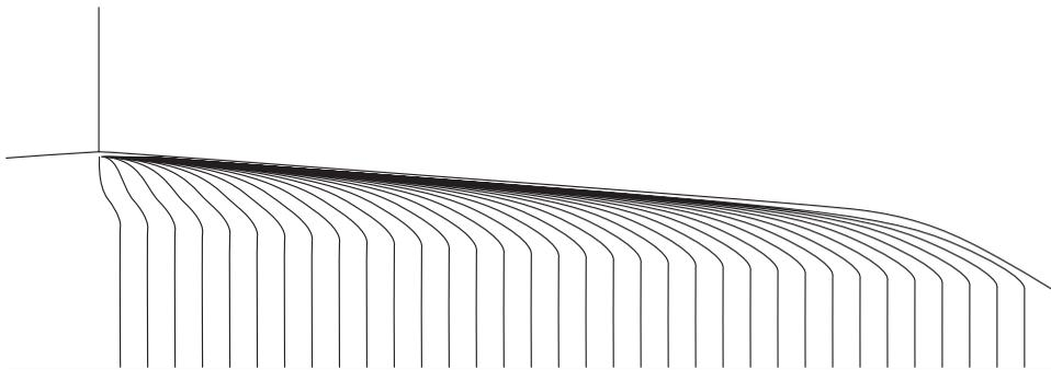
**Figure 4.13** Streamlines predicted by the FLATCAD ADVANCE software package [28], for the die geometry shown in **Figure 4.12**
