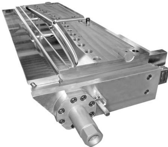
**Figure 4.6** Picture of the lower half of a modern flat die having a lower sliding lip, which can be adjusted during production. Reproduced with permission from EDS GmbH, Kirchdorf, Austria
