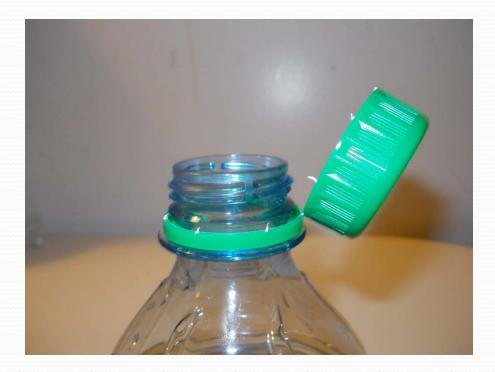
It was impossible to mold twist-off caps with a new PE grade, at a large corporation
