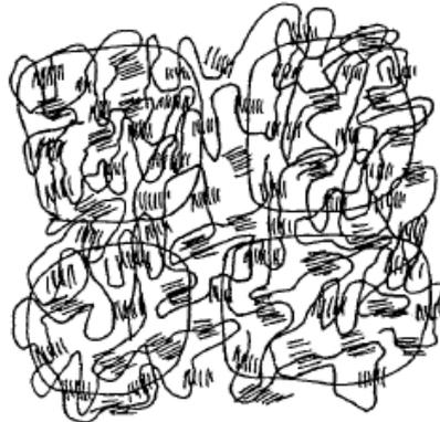
c) Partially melted then recrystallized high molecular weight PVC, showing strong three dimensional structure.
