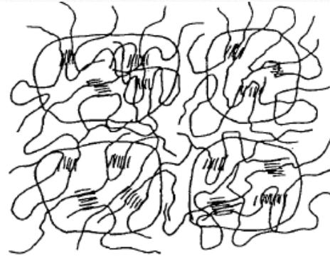
b) Partially melted PVC primary particles.
