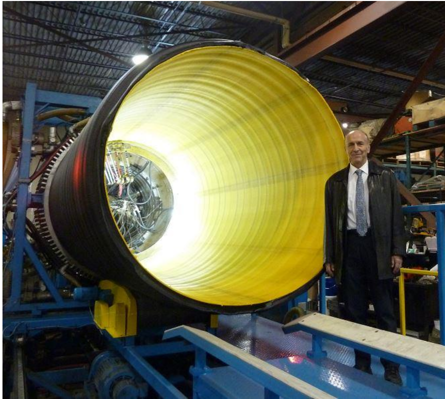
Fig. 5 Production of double-wall corrugated pipe
