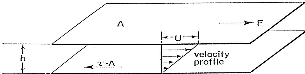
Figure 1.1. Simple shear flow.
