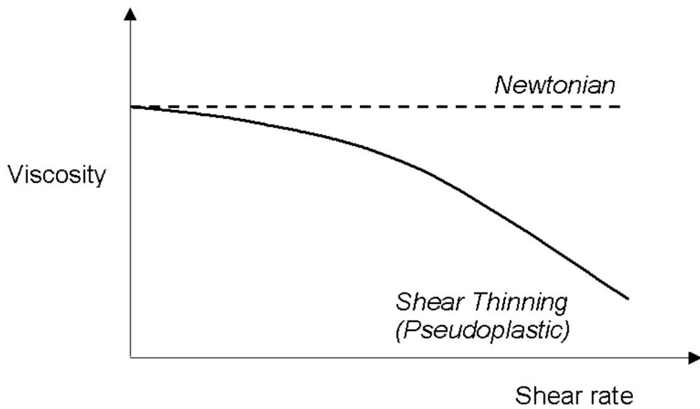
Figure 1.3. Newtonian and shear-thinning viscosity behavior.
