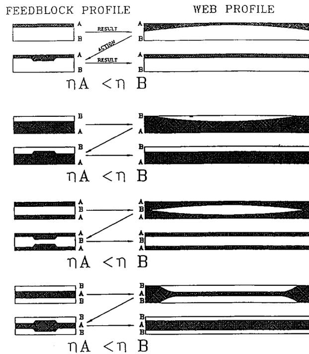
Figure 1.14. Feedback profiling and the resultant effects.
