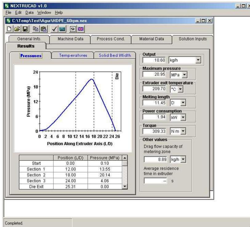
Figure 1.16. Simulation prediction of pressure build-up in extruder.
