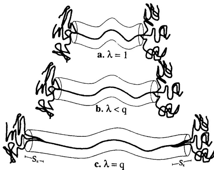
The structure of a pom-pom polymer with a backbone and  $2q$  dangling arms, with  $q = 3$ , under various degrees of stretch. The stretch of the backbone is denoted by the variable  $\lambda(t)$ , the path length of arm withdrawn into the backbone tube by the variable  $s_c(t)$ .
