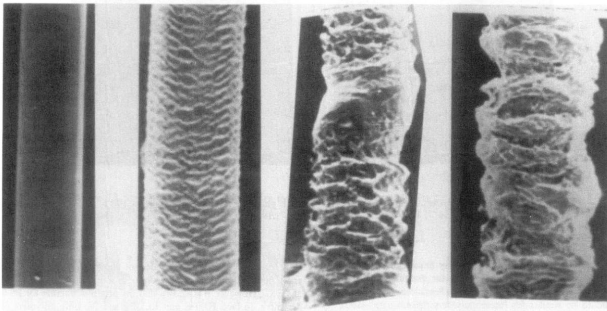
Figure 1.12. LLDPE extrudates obtained from a capillary at apparent shear rates of 37, 112, 750 and  $2250 \text{ s}^{-1}$ .
