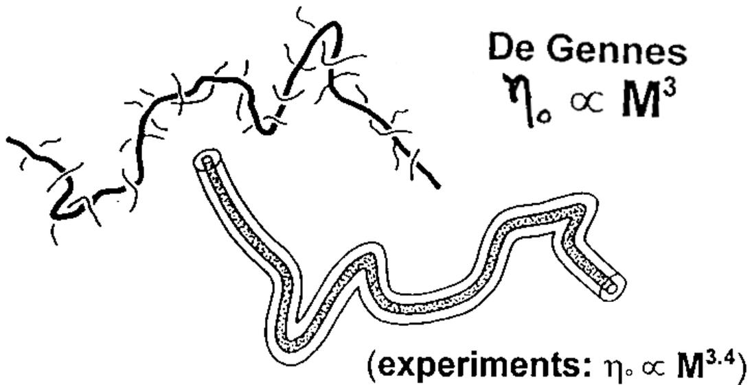
Figure 1.10. Reptation model of polymer chain motion.
