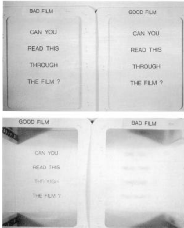
Figure 1.15. The effect of interfacial instability on contact clarity of coextruded films (top) versus see-through clarity (bottom).
