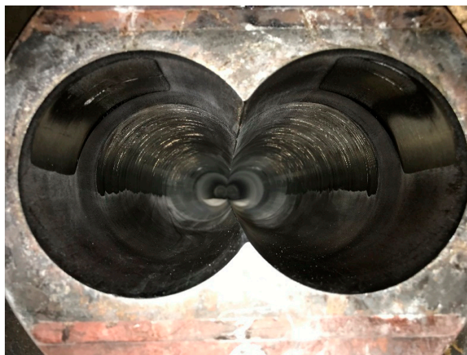
Figure 2. Wear in a nitrided parallel twin barrel, 90 mm screw diameter, 26 L/D ratio. It was run with a highly filled PVC formulation for more than 10,000 h. Highest wear seems to be between the 30° and 60° angle from the vertical.
